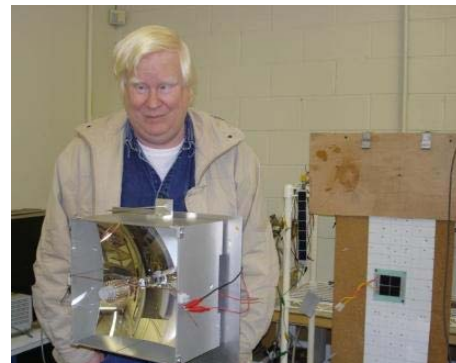
Dr. Fraas with a Cassegrainian prototype solar module. This module concentrates 500 times more sunlight on each solar cell.
