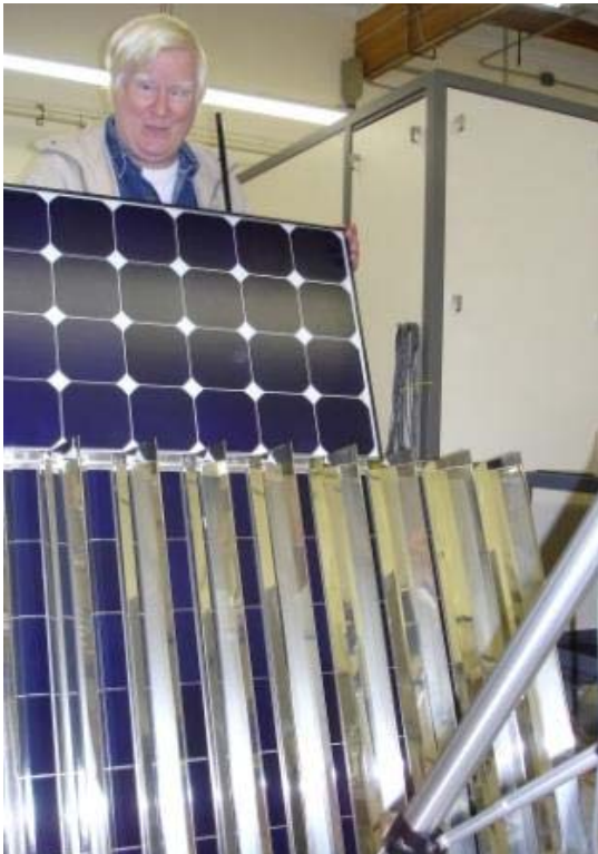
The mirrors on the 3-Sun module below allow much more PV power to be produced with fewer solar cells.
