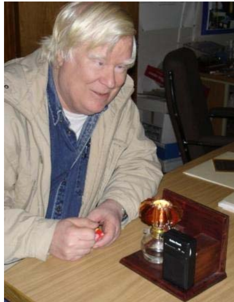
Dr. Fraas with thermophotovoltaic lamp. Tiny TPV crystals turn infrared energy in the flame into electricity to power a tiny radio.
